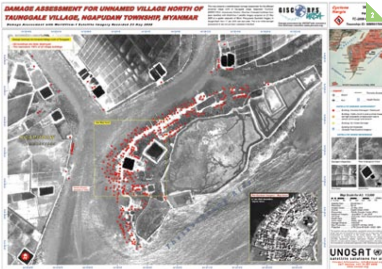
▲ FIGURE 2. Overview of 18 villages affected by Myanmar cyclone, a final online deliverable made available to relief workers using a combination of remote sensing sources and attributes generated by GISCorps volunteers as a Landat Mosaic (ESRI-MDC). Damaged buildings have been identified with WorldView-1 satellite imagery (DigitalGlobe) acquired on May 6, 8, 10, 23 and 27, 2008 at a spatial resolution of 50 cm. Pre-cyclone Quickbird imagery from 2005 was also used for change detection. Processing by Pacific Disaster Center. Image courtesy of GISCorps, NGA, Respond/Keyobs.
