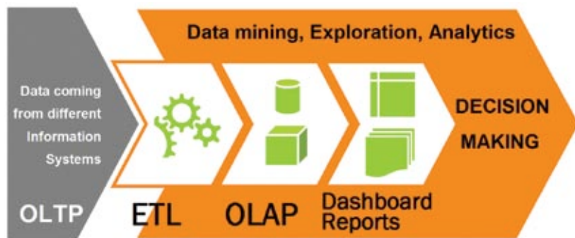
▲ FIGURE 1. This figure is a technical illustration of what needs to happen behind the scenes (handled either by your IT department or by a managed service) to convert transactional data sources, such as stats, logs, CRM, ERP, etc., known as an OLTP (Online Transaction Processing) data model, to an analytical format that can then be used by an analyst, manager, or executive in the form of a data-mining or dashboard application. Transactional data must go through an ETL (Extract, Transform and Load) tool, which is able to properly feed a data warehouse in a specific OLAP data model. Graphic courtesy of Spatialytics.
