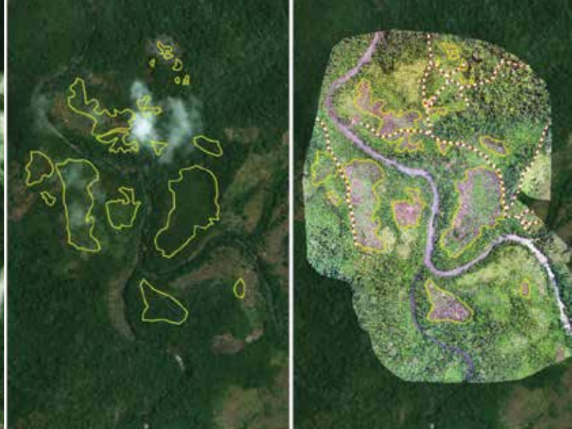
Figure 6. UAVs were used to document illegal deforestation and road building in Majé Emberá lands. On the left is 2016 imagery from ArcGIS Online, with polygons showing the forest cover lost by May 2018. The right image is UAV images from May 2018 verifying the deforestation and roadbuilding.
