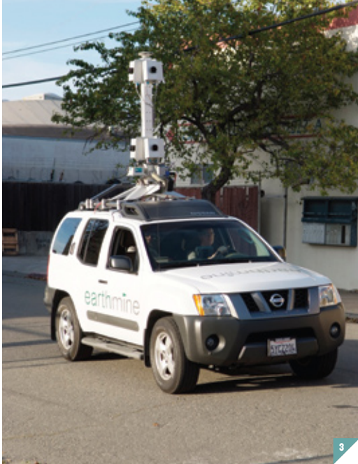
◀ FIGURE 3 earthmine's mobile stereo panoramic collection system drives and scans hundreds of miles a day.
