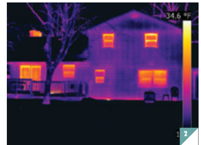
► FIGURE 1 Airborne Thermal IR of homes, depicting energy loss differences with 25-cm ground resolution at 1000-meter altitude (courtesy of Jenoptik).
