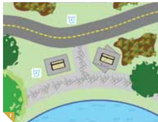
▲ FIGURE 6. Using a template for park features that utilizes cartographic representations and a reference scale on the map, you can draw features in real-world distances. Trees and trail widths are consistent with your design specs, giving an instant visualization of the layout of the park.
