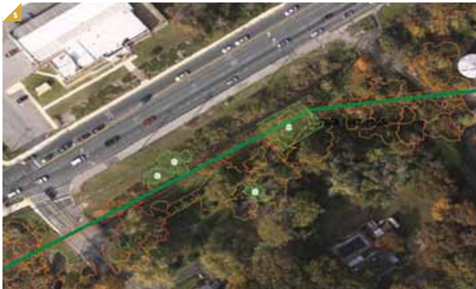
◀ FIGURE 5. An image generated in GeoDigital's VegWorks mobile work management software reflects asset and all related field data including poles, spans, maps, aerial photography, LiDAR mapping, customer information and work history. The application merges the data to allow a utility to quickly identify any right-of-way threats and to produce all work order details to dispatch crews for remediation.
