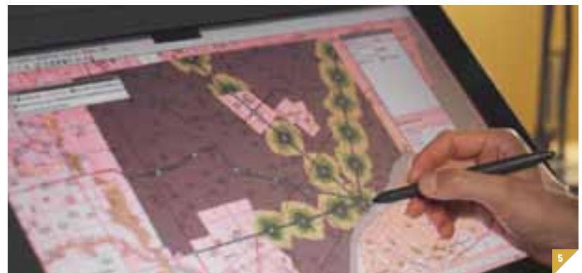
▶ FIGURE 5. This light-rail planning sketch ties into the underlying road network giving a walkability map of the light-rail stops. This gives a visualization of the ¼, ½, and 1 mile walkability radius along the road network, i.e. what areas are well served by the light-rail stations. This can then be used to find areas suitable for re-development.
