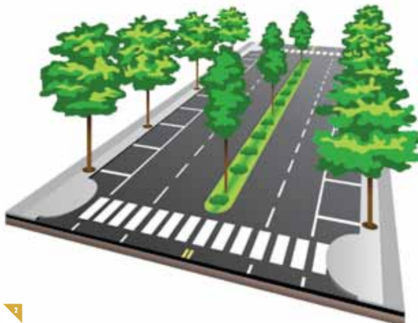
▲ FIGURE 2. A four-lane boulevard with traffic calming features and bioswale for a median.
