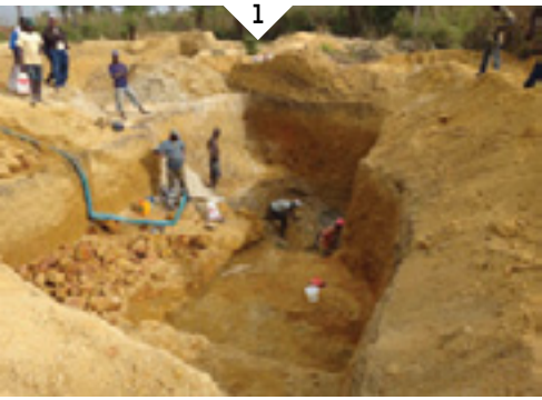
▲ FIGURE 1. A typical artisanal mining site: Workers begin mining in an area by digging a cluster of exploration holes until the presence of a thick and potentially rich gravel layer is found in the alluvial floodplain. Miners will then dig through several meters of sandy overburden material to access the diamondiferous gravel layer deep in the floodplain. When the gravel layer is reached, miners extract the ore and carefully sort and wash it in search of diamonds. This washing and sorting activity is completed within the active pit itself, in an adjacent pit that has filled with water, or in a nearby stream. It typically takes a team of three men one to three weeks to dig a pit, extract the gravel, and sort it for diamonds. Once the process is complete, the miners begin a new pit. Rarely, if ever, do the miners fill in previously mined pits. Old pits therefore remain exposed and typically fill with water. Photography courtesy of Peter Chirico, USGS.
