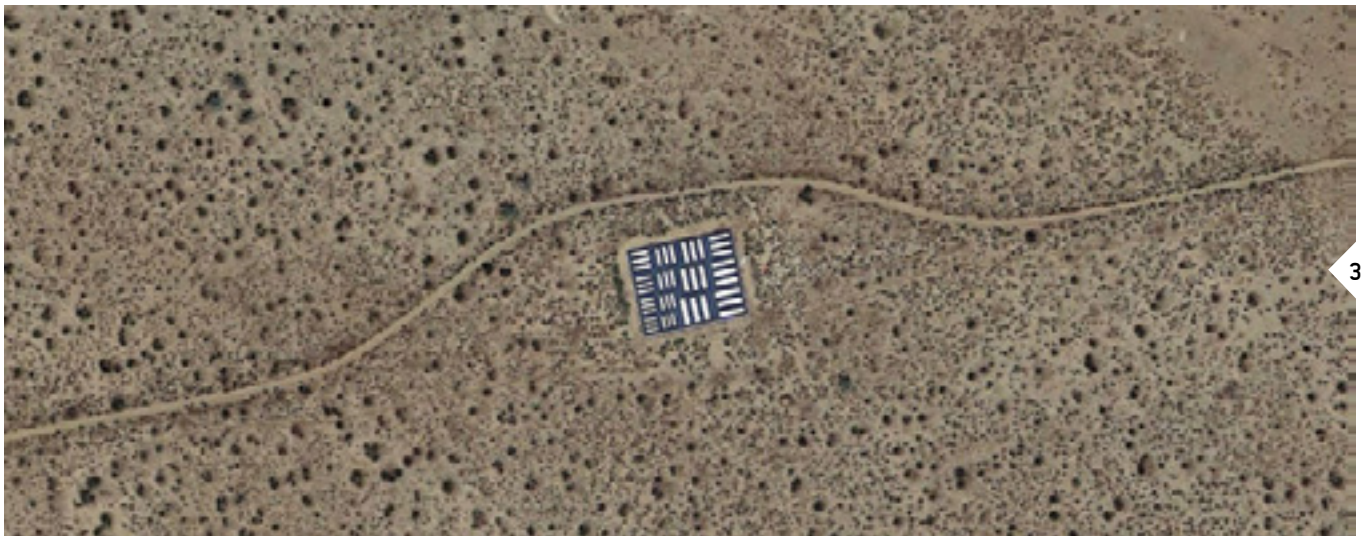
▲ FIGURE 3. The aerial sensor calibration site located at Edwards Air Force Base in California (Google Earth Image)
